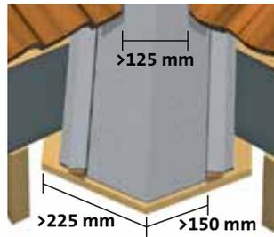
When the tiles/slates are laid the gap between them should not be less than 125mm. Valley boards (not less than 19mm thick) are laid on top of the rafters in boarded
