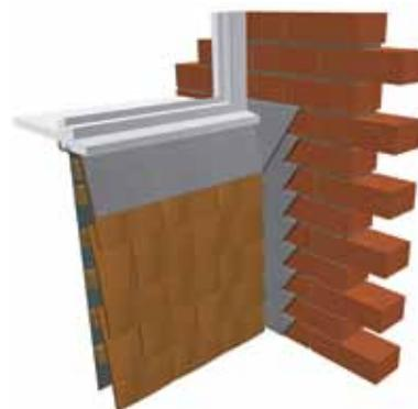
Figure 10: flashing to vertical tile or slate hanging – cills
