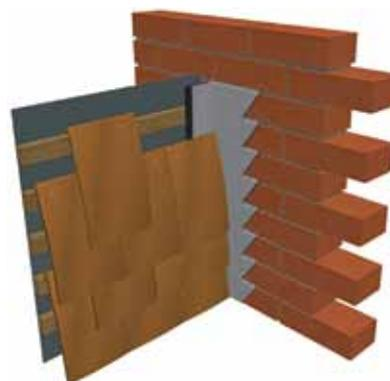
Figure 9: flashing to vertical tile or slate hanging – side abutment
