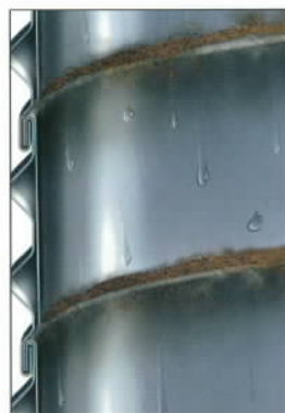
Conventional folded seam joints can loosen under compressive loads permitting condensates to enter.
